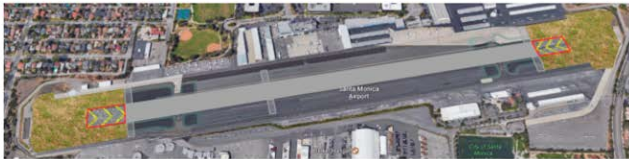
The green/yellow areas at each end of the runway depict the area where the excess pavement will be removed and replaced with grasses and plants.
